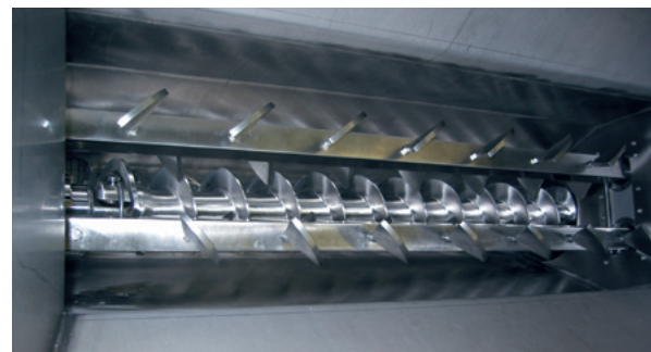
View inside the hopper with adjustable paddles above the conveying screw
