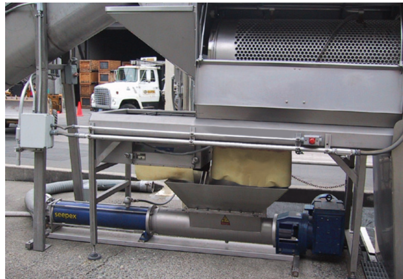
Beaulieu’s BT 130-6L open hopper must pump sits beneath the destemmer, ready for another harvest season
