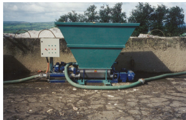
... and transported into a mobile soil injection unit by a seepex BTI range pump.
