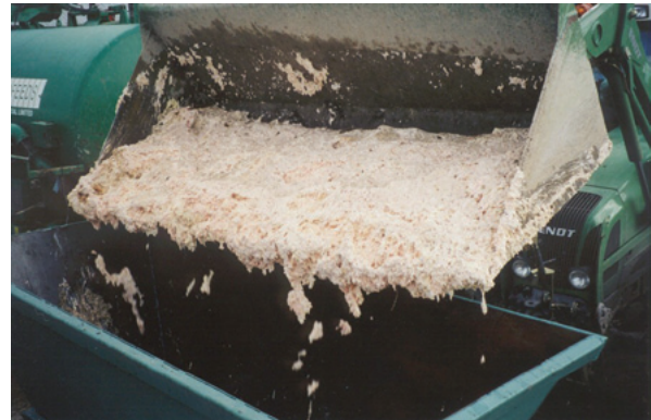
The waste is loaded into the hopper above the pump ...
