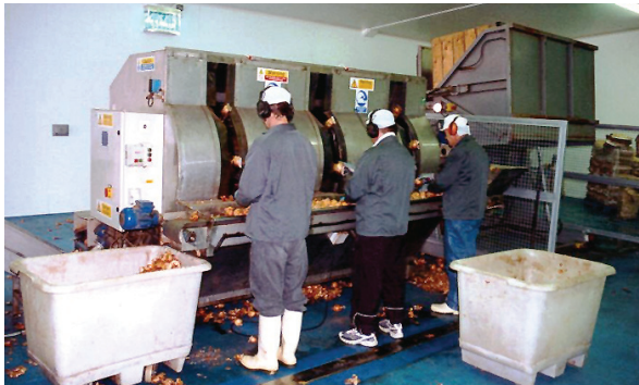
Onions being placed into peeling machine
