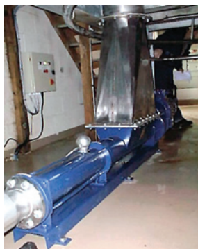
seepex BT range pump while conveying spent grain out of the mash tun into a tractor-trailer
