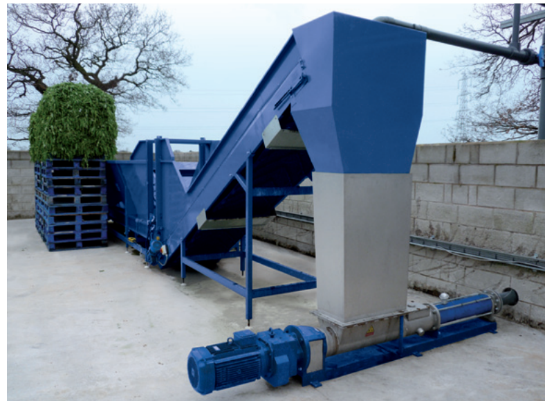
seepex BTM range pump chops and transports tomato vines in a single step
