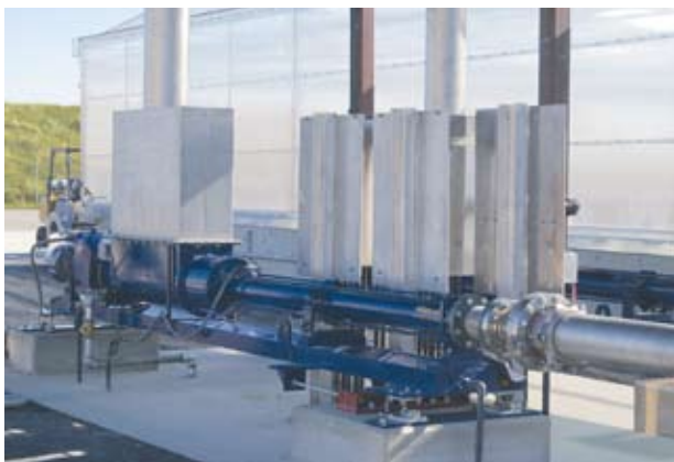
Pumps of range BTHE 70-24 with hopper level controlled via load cells Conveying product: Dewatered sludge with a ds content of up to 20 – 35 % Conveying capacity: 10 m 3 /h (44 GPM) • Pressure: 14 bar (203 PSI) Temperature: 20 °C (68 °F)
