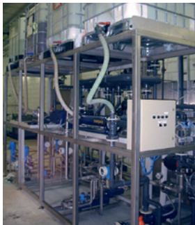
seepex BN range pumps convey ingredients for cosmetics into a mixing system
